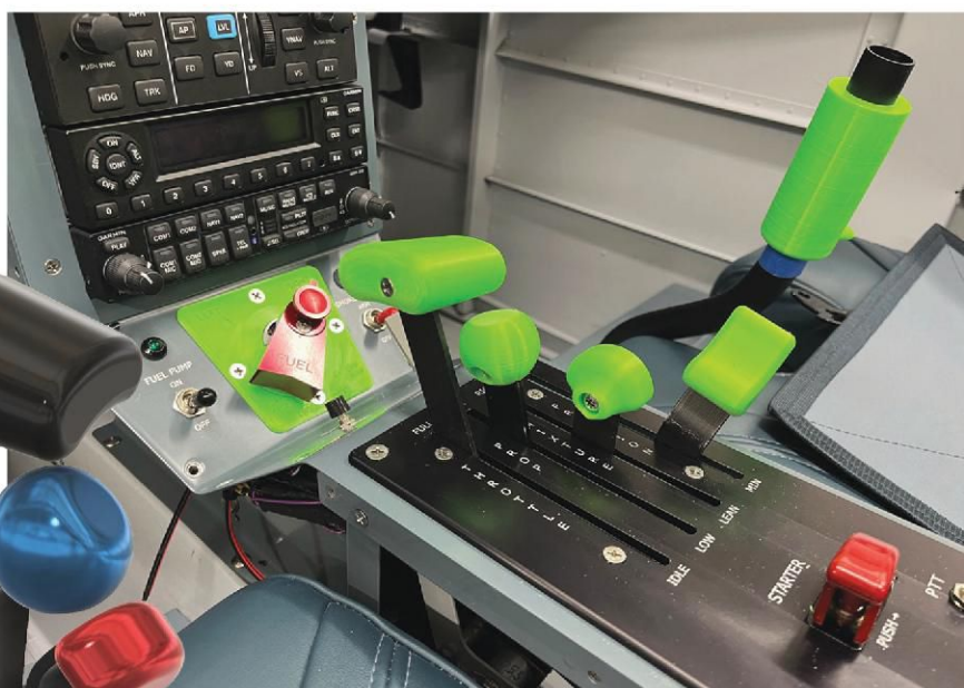
3D-printed knob prototypes in place for review
